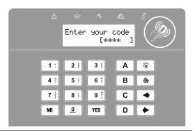
The alarm symbol will flash indicating there has been an alarm activation and the keypad will display which input has activated.
